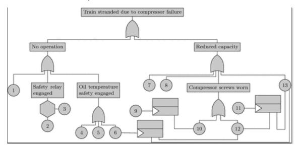
Figure 4.9: The fault tree used in the study of Ruijters et al (2006)indicates the major failure modes of the compressor.
