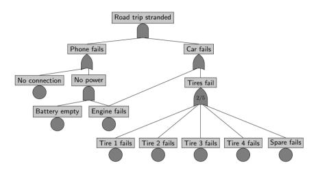
Figure 2.2: An example of a fault tree.
