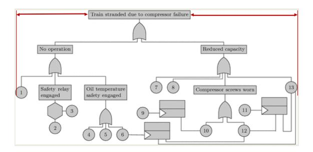
Figure 4.12: The fault tree is not organized symmetrically
