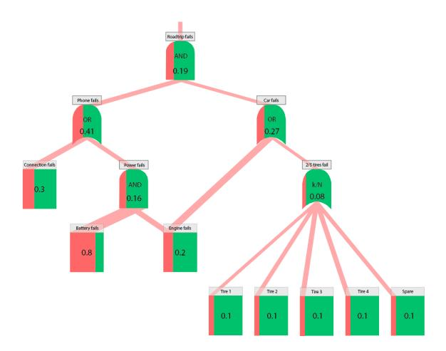
Figure 17: The hybrid fault tree concept
