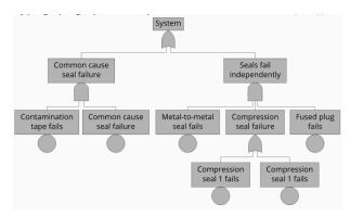
Figure 1: An example of a fault tree [4]
