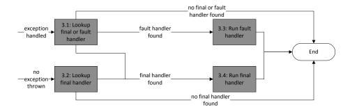
Figure 3.5: Flow diagram of finalising mode.
