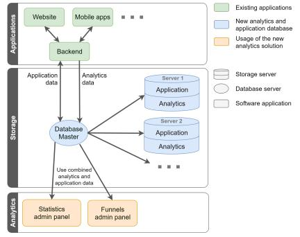
Figure 5: Usage and profile data storage architecture
