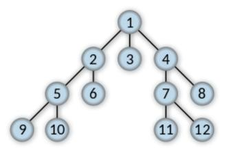
Figure 2.1: Order of traversal for BFS, where the top vertex is the source
