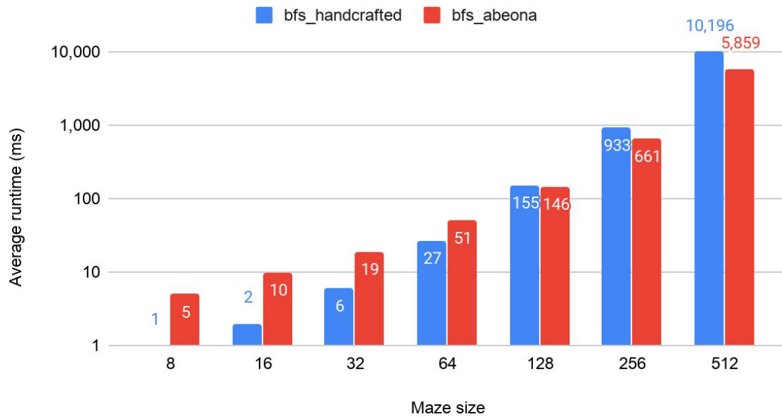
Figure 5.3: Runtime comparison of a handmade BFS algorithm (blue) against a composed query in Abeona (red) for various sizes of mazes.
